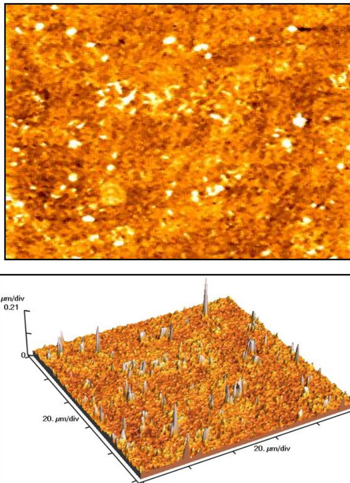
Fig. 3 Atomic force microscopy (AFM) images for SnO<sub>2</sub> 20% F-doped.
