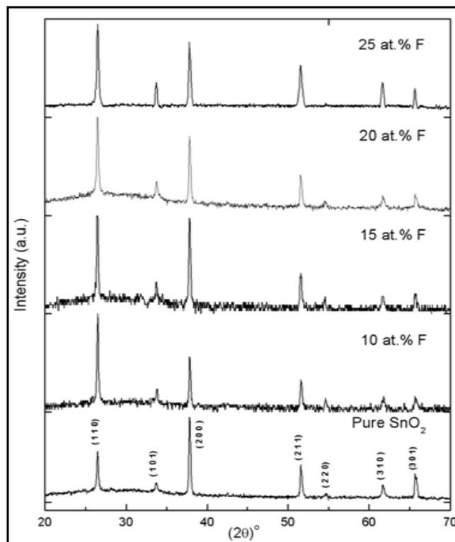
**Fig. 1** x-ray diffraction (XRD) patterns of pure and doped SnO<sub>2</sub> with different concentrations of fluorine (a): pure, (b):10%, (c): 15%, (d): 20% and (e): 25%.
