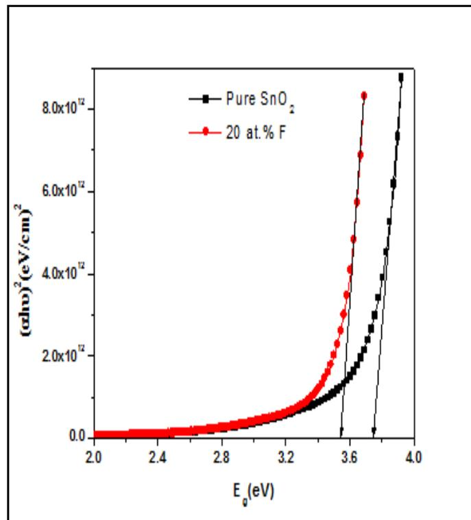
Fig. 5 change of band gap position for SnO<sub>2</sub> thin films doped with 20at. % F.
