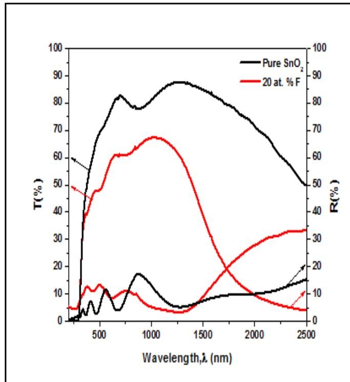
Fig. 4 optical transmittance & reflectance spectra of pure and 20at. % F-doped SnO<sub>2</sub> thin films
