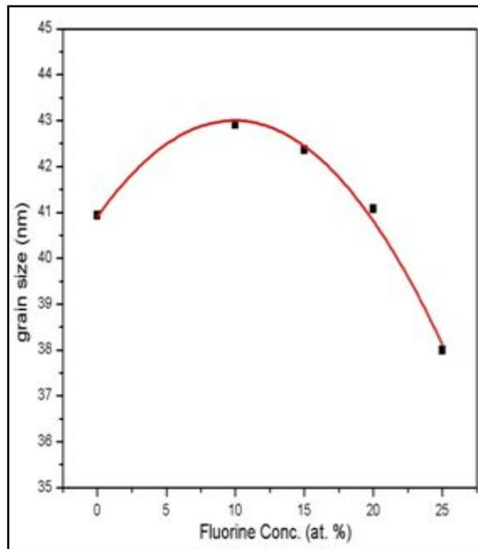
Fig. 2 the effect of fluorine concentration on the crystallite size.
