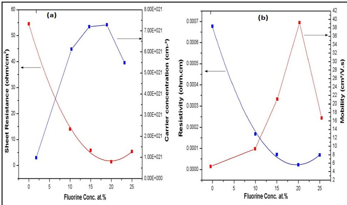
Fig. 6 sheet resistance, carrier concentration, resistivity and Hall-mobility of sprayed SnO<sub>2</sub>: F versus the Fluorine concentration.
